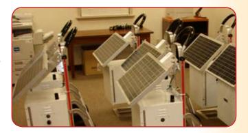
Seismic Survey has built "seismo-bots" which work in conjunction with modems and InstaLink to monitor several remote projects without having staff on site.
